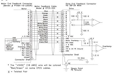
Figure 15: Motor Feedback Connector Pinout
